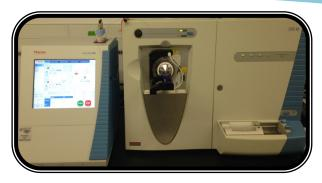
A top notch **Easy-nLC 1000** couple to **LTQ XL** mass spectrometer from Thermo Scientific is available and configured for maximum coverage in protein identification. Nanoflow LC is optimized for separating peptides at ultrahigh pressures.
