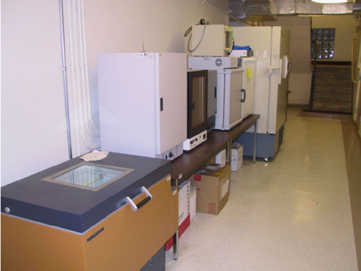
6. Biofreezer and incubators in the facility hallway
