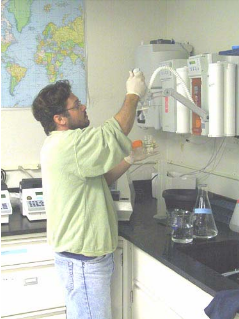
3. Lab technician Luis Quiñones drawing "holy" water from the Milli-Q Synthesis system
